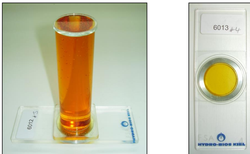
Figure 28: Phytoplankton cells in a 50 mL sub sample of Lugol's-fixed seawater are allowed to settle onto the base plate of the chamber prior to analysis.
