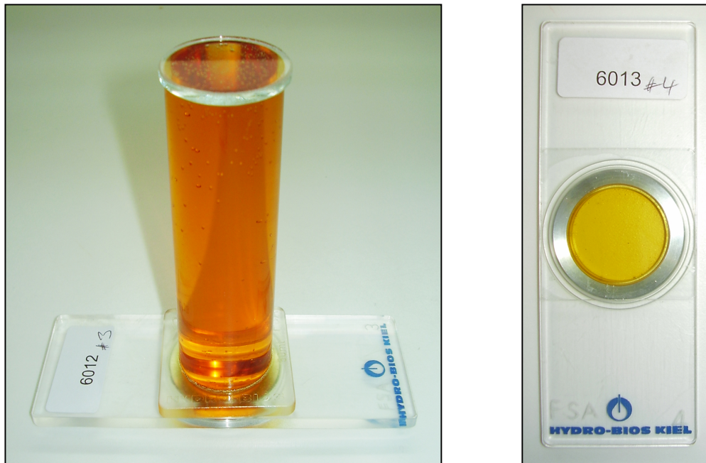
Figure 27: Phytoplankton cells in a 50 mL sub sample of Lugol's-fixed seawater are allowed to settle onto the base plate of the chamber prior to analysis.
