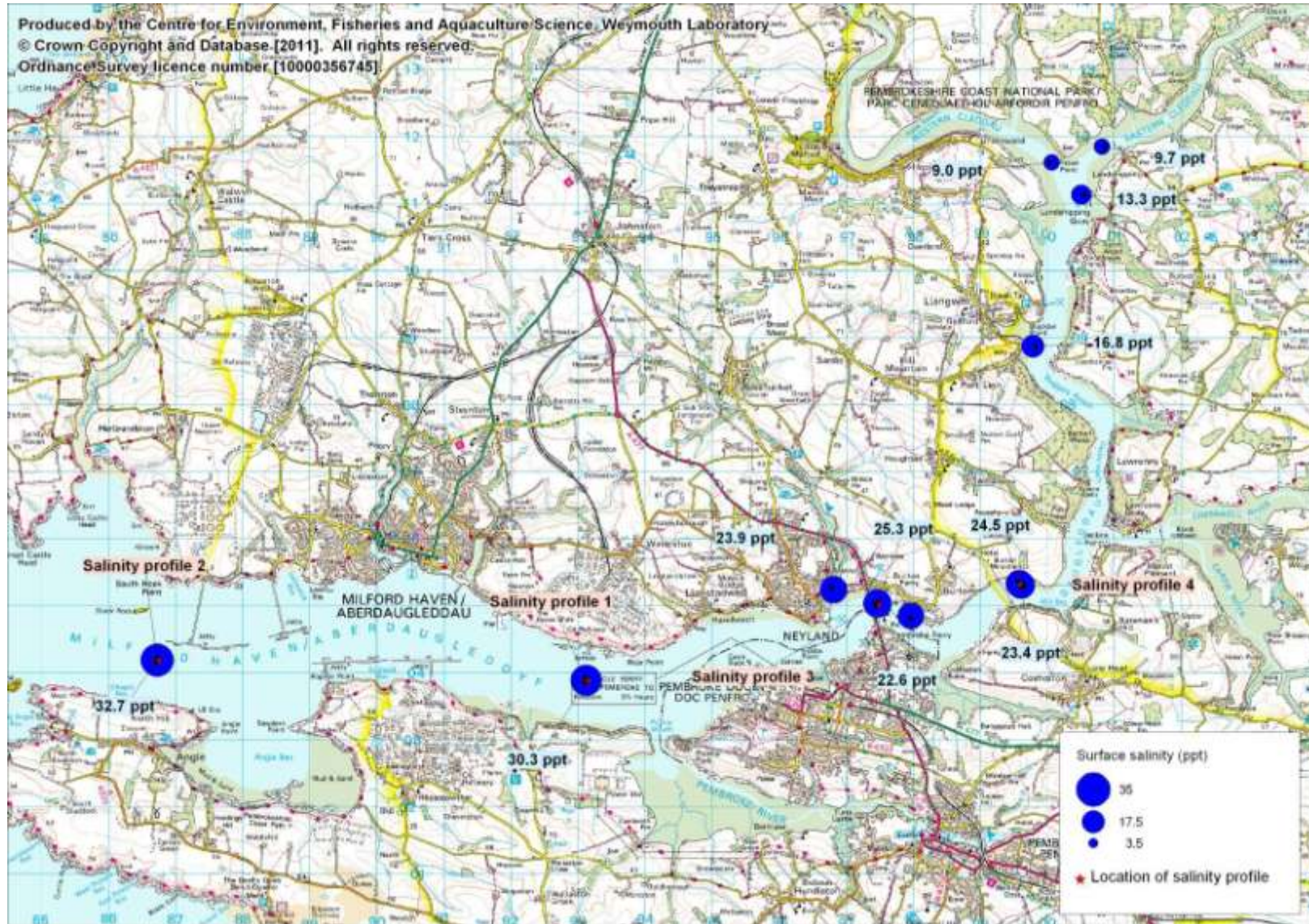
Figure XIII.3. Thematic map of surface salinity measurements and location of vertical salinity profiles
