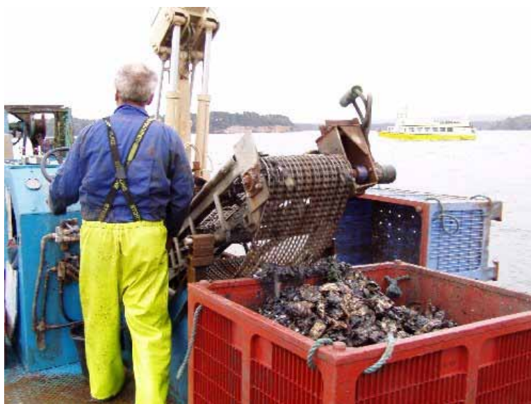
Figure 3.2 Harvesting Pacific oysters in Poole Harbour on conveyor harvester. Photo courtesy of Gary Wordsworth, Othniel Oysters Ltd.
