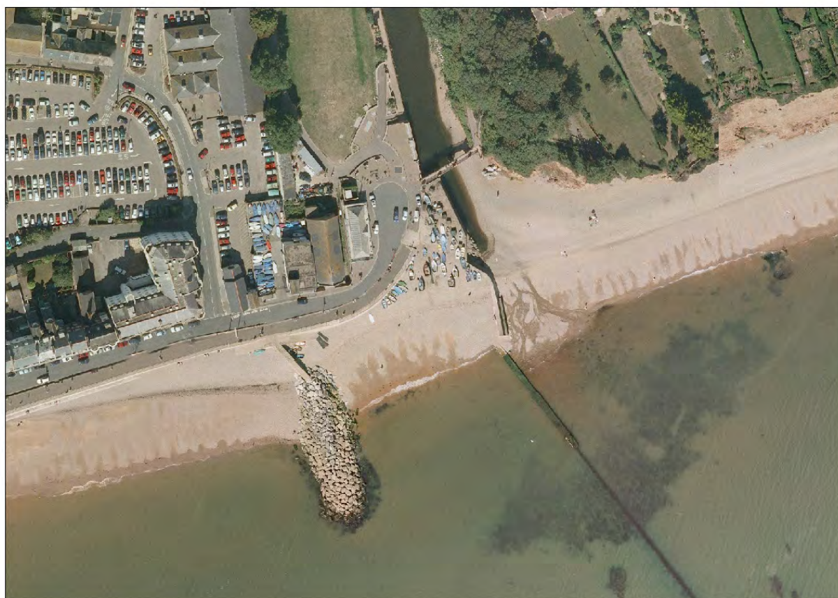
Figure 3.3: Mouth of the River Sid at low flow. Note the channelised lower river course, the river flow through the beach and the river training wall to the west of the river mouth. Image courtesy of Channel Coastal Observatory ( www.channelcoast.org ).
