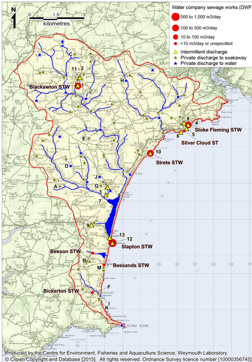
Figure II.1: All permitted sewage discharges to the Start Bay catchment Contains Environment Agency information © Environment Agency and database right
