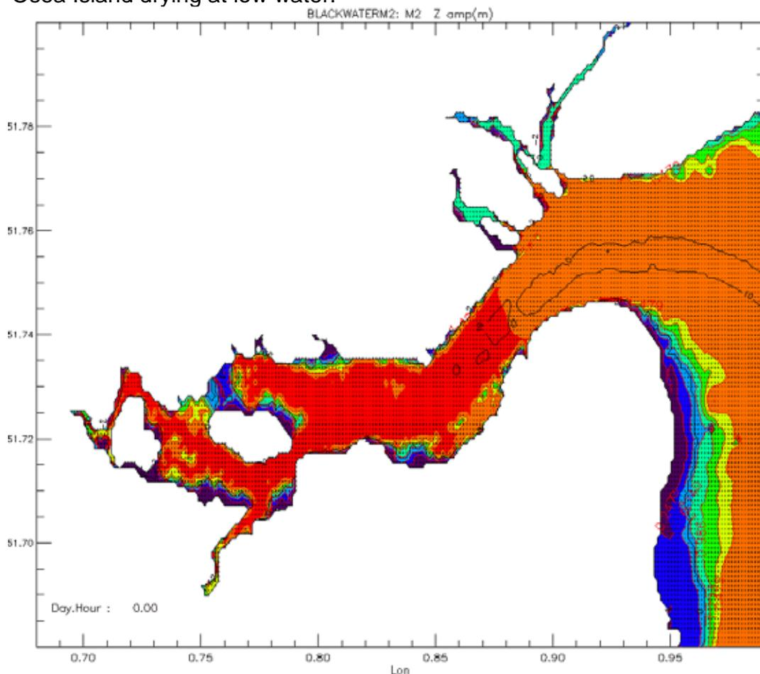
**Figure V.1 Surface elevation tidal amplitude in the Blackwater Estuary.**
