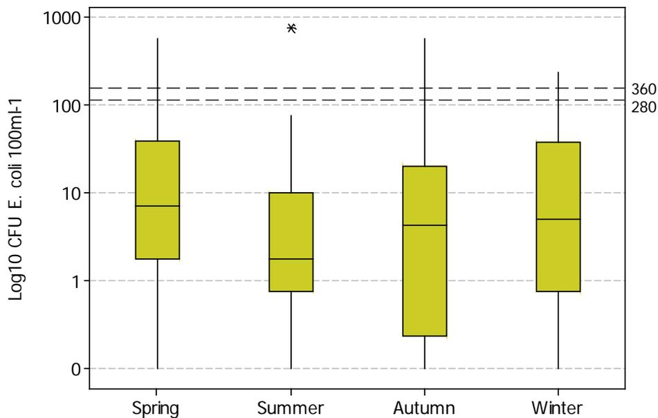
**Figure VII.2 Box-and-whisker plots of seasonal levels of faecal coliforms in the final effluent post UV disinfection monitored in West Mersea sewage treatment works.**
