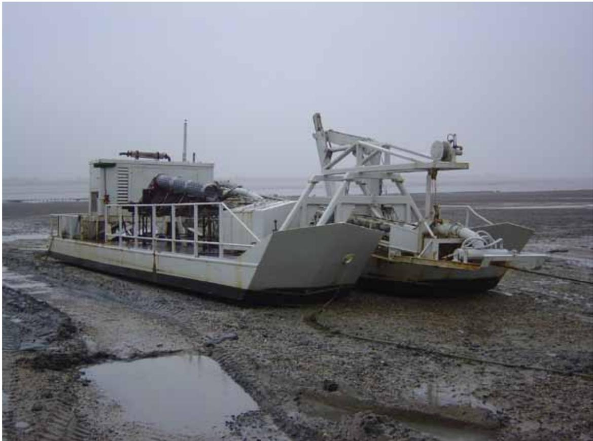
*Figure 2.3 Vessel used for dredging shellfish in the Blackwater Estuary.*
