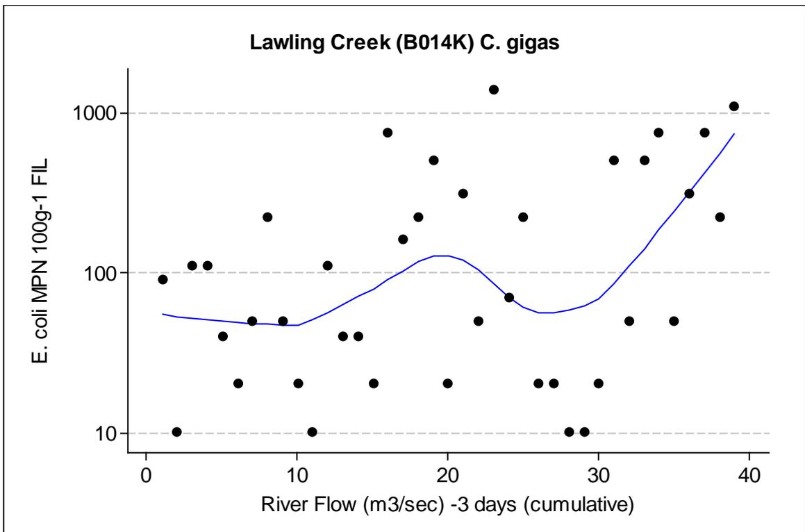
**Figure XII.5** Scatterplot of levels of *E. coli* at Lawling Creek versus cumulative river flow recorded at Langford for three days previous to sampling for the period April 2003–March 2009.
