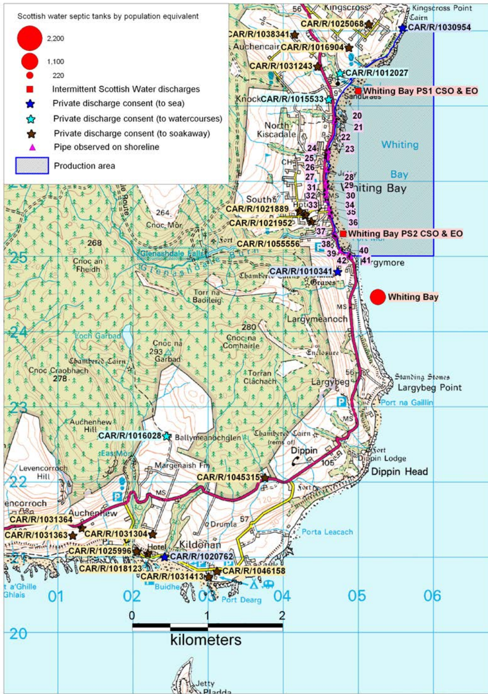
Figure 4.3 Sewage discharges at Whiting Bay (south of Kingscross Point)
