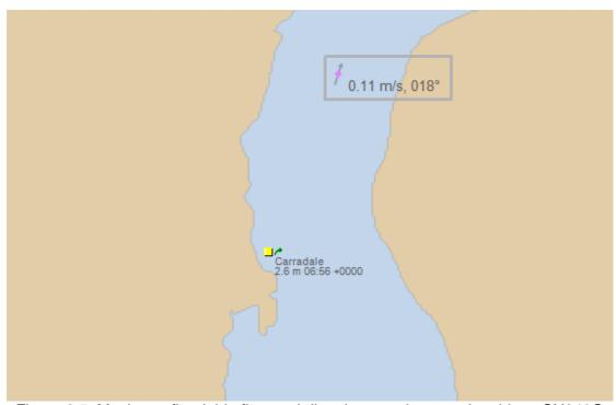
Figure 8.5 Maximum flood tide flow and direction on a large spring tide at SN040G (from Admiralty TotalTide)
