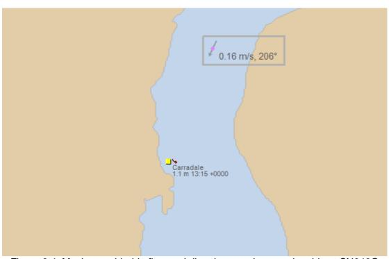
Figure 8.4 Maximum ebb tide flow and direction on a large spring tide at SN040G (from Admiralty TotalTide)
