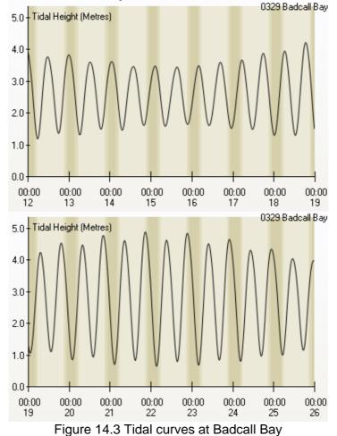
The two tidal curves illustrated in Figure 14.3 are for Badcall Bay on the eastern side of Eddrachillis Bay. The tidal curves have been output from UKHO TotalTide. The first is for seven days beginning 00.00 BST on 12/08/09 and the second is for seven days beginning 00.00 BST on 19/08/09. This two-week period covers the date of the shoreline survey. Together they show the predicted tidal heights over high/low water for a full neap/spring tidal cycle.
