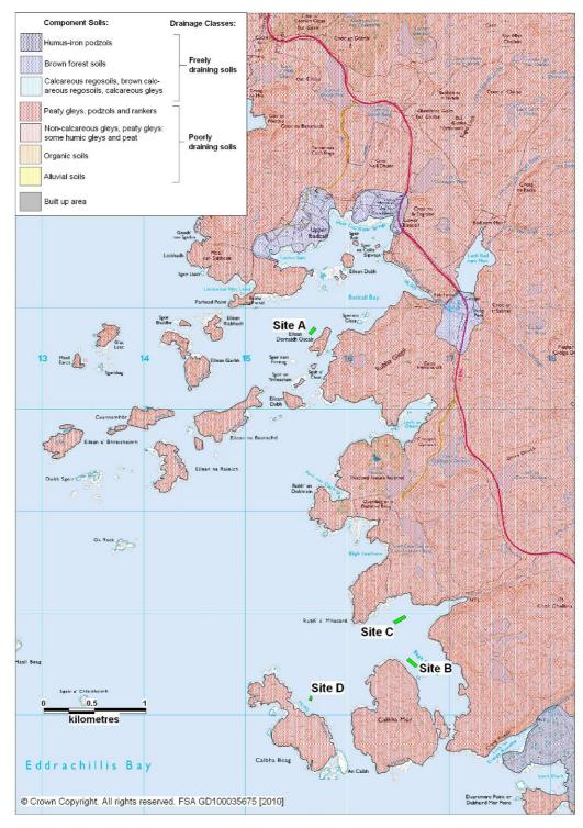
Figure 5.1 Component soils and drainage classes for Badcall/Eddrachillis Bay
