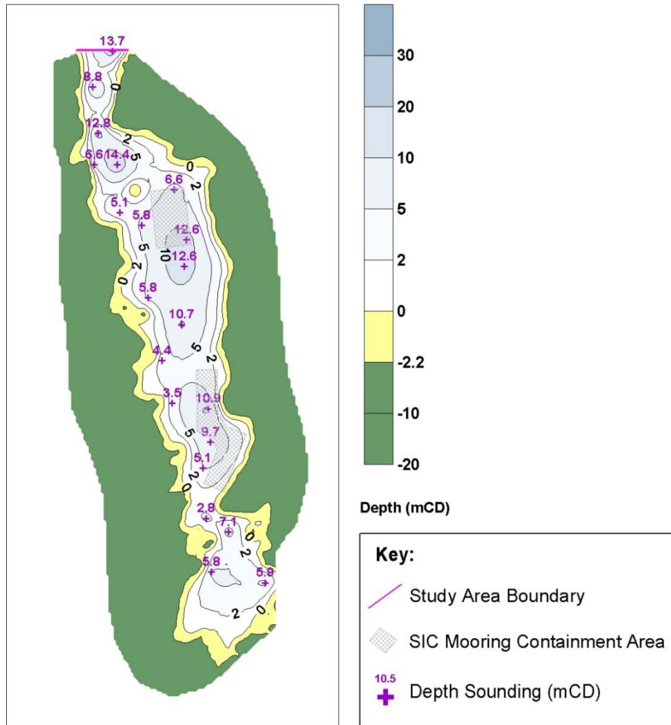
Depths corrected to metres chart datum. MLWS and MHWS data extracted from Ordnance Survey Explore Sheet 467
