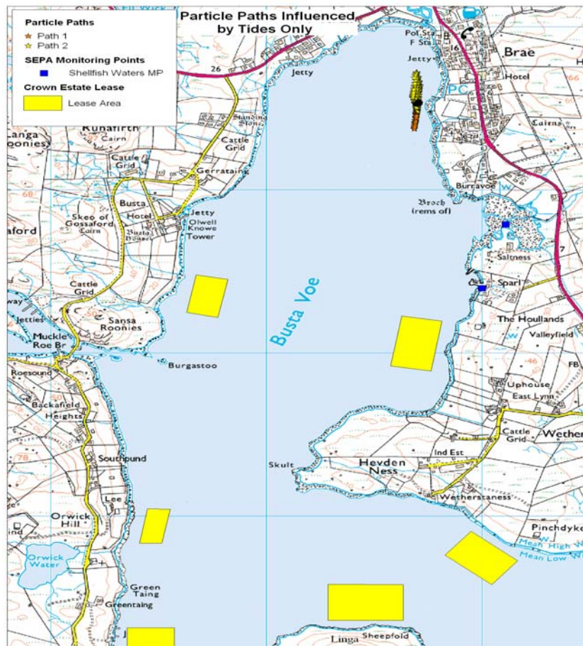
Figure 13.3: Particle paths for tide only. The black circle shows the start location. Two paths are shown representing particles released on flood and ebb tides. (about 6.2 hours apart).
