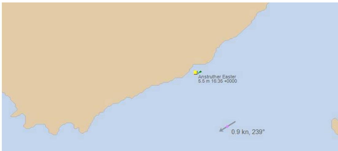
Figure 8.5 Maximum flood tide flow and direction on a large spring tide at SN022A (from Admiralty TotalTide)
