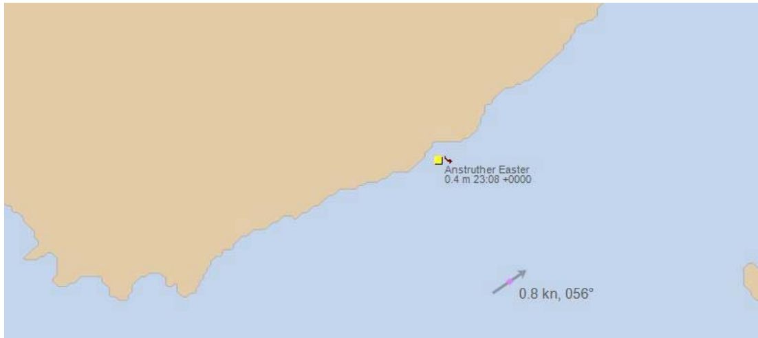
Figure 8.4 Maximum ebb tide flow and direction on a large spring tide at SN022A (from Admiralty TotalTide)
