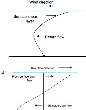
Figure 1. Typical vertical profiles for water currents. The black vertical line indicates zero velocity so portions of the profile to the left and right indicate flow moving in opposite directions. a) Peak tidal flow profiles. Profiles are shown 6.2 hours apart as the main tidal current reverses direction over a period of 6.2 hours. b) wind driven current profile, c) density driven current profile.
