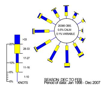
Figure 9.6 Wind rose for Tiree (December to February) Figure reproduced under license from Meteorological Office. Crown Copyright 2010.
