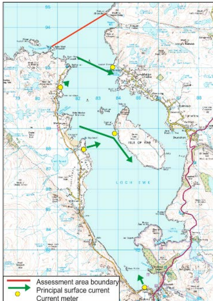
Figure 13.4 Map showing Loch Ewe ADCP and current meter sample sites within the assessment area. Using the surface principal current amplitude and the assumption of a uniform sinusoidal tide, the cumulative transport distance and direction that might be expected during each phase of the tide is shown above.
