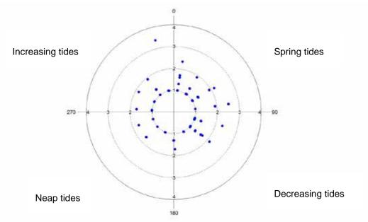
Figure 11.13 Polar plots of log<sub>10</sub> *E. coli* results at Loch na Keal West against the spring/neap tidal cycle
