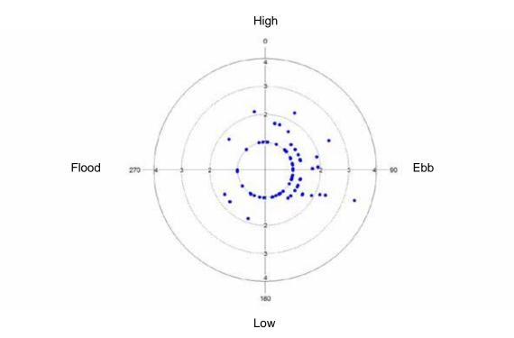
Figure 11.15 Polar plots of log<sub>10</sub> *E. coli* results at Loch na Keal West against the high/low tidal cycle
