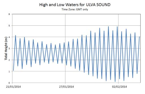
Reproduced from Poltips3 [www.pol.ac.uk/appl/poltips3] Figure 13.3 Two week tidal curve for Ulva Sound, Loch na Keal.
