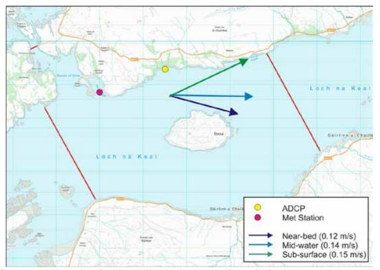
Figure 13.4 Map showing Loch Na Keal sample sites within the assessment area. Using the principal current amplitude at each measured depth and the assumption of a uniform sinusoidal tide, the cumulative transport distance and direction that might be expected during each phase of the tide is shown above. Residual transport was determined to be negligible.
