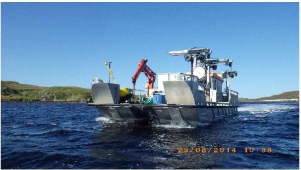
**Fig 6**: Aluminium mussel farm harvesting vessel – photo taken on passage in Loch Barraglom on return to shore base.
