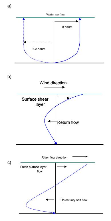
Figure 1. Typical vertical profiles for water currents. The black vertical line indicates zero velocity so portions of the profile to the left and right indicate flow moving in opposite directions. a) Peak tidal flow profiles. Profiles are shown 6.2 hours apart as the main tidal current reverses direction over a period of 6.2 hours. b) wind driven current profile, c) density driven current profile.
