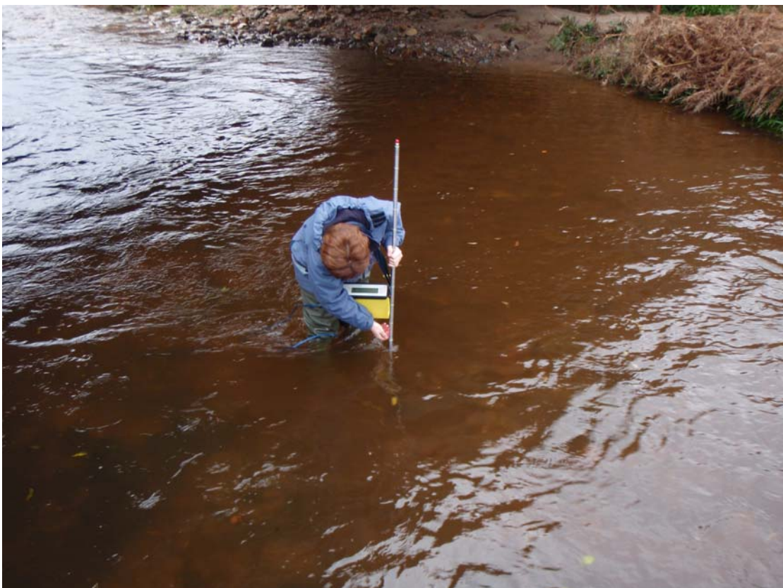
Figure 24. Measuring flow in large burn
