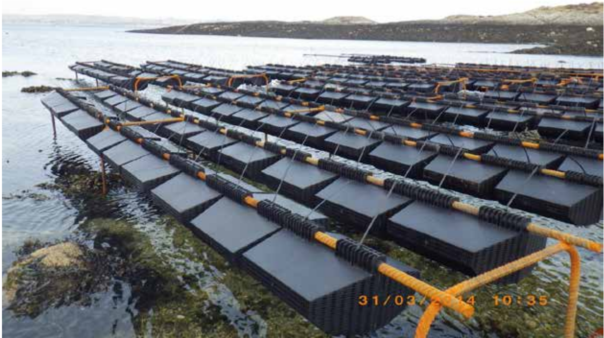
Figure 9. Corner of trestles with new Ortac box system at the middle of shellfish site. Waypoint 21.
