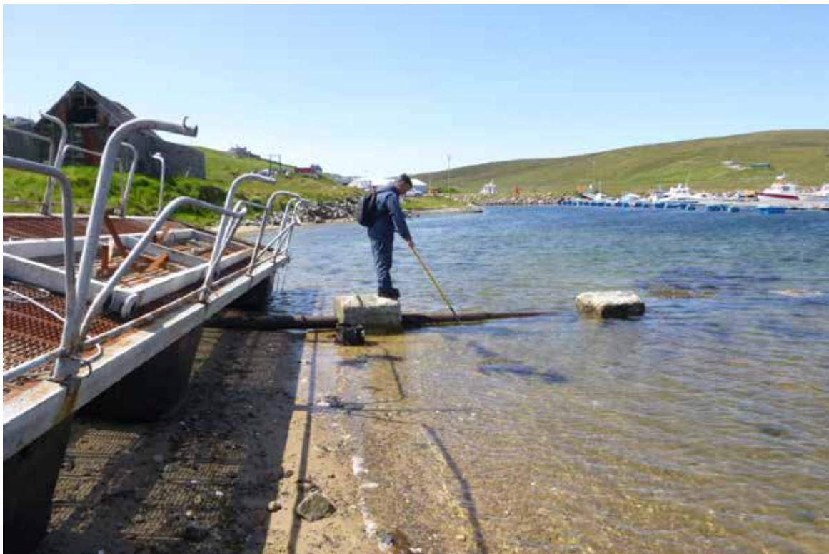
Figure 7 – Sea water sample being obtained near the Ravensgio Septic Tank discharge pipe.
