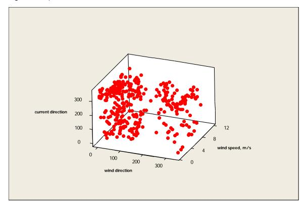
Figure 14.5 Near-surface current direction versus wind speed and direction
