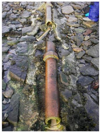
Figure 17. Broken pipe, fresh water sample 7
