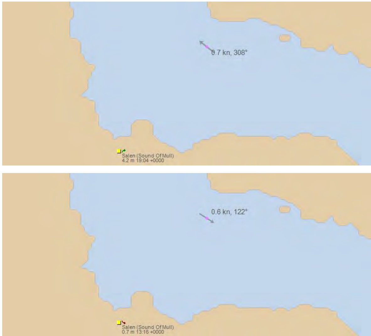
Figure 13.4. Tidal flows and direction at peak flow during a spring tide on the flood tide (top) and the ebb tide (bottom) at SN037B (taken from TotalTide)
