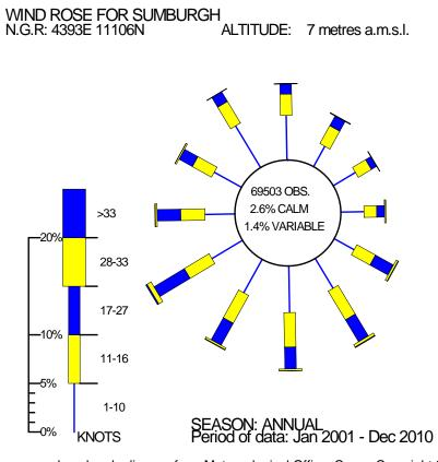
Figure reproduced under license from Meteorological Office. Crown Copyright 2012. Figure 9.4 Annual wind rose for Sumburgh
