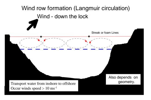
Figure 2. Schematic of wind driven 'wind row' currents. The dotted blue line indicates the depth of the surface fresh(er) water layer usually found in sea lochs.
