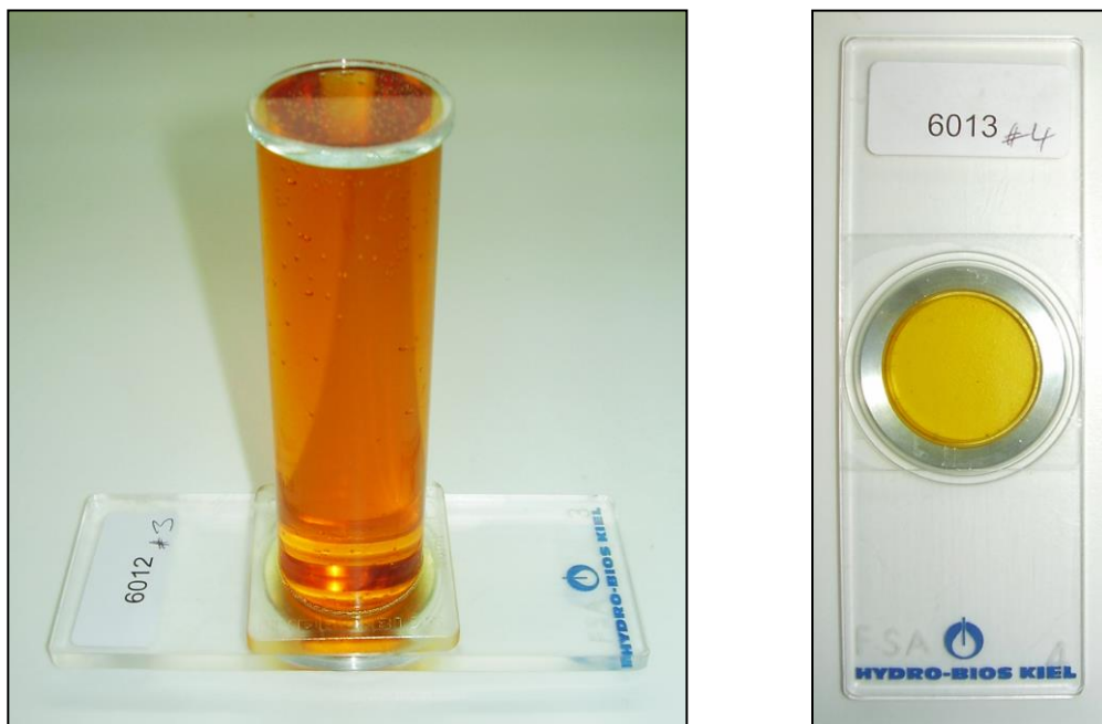
Figure 28. Phytoplankton cells in a 50 mL sub sample of Lugol's-fixed seawater are allowed to settle onto the base plate of the chamber prior to analysis
