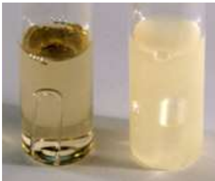
Figure 1. A negative (no growth) and positive (growth accompanied by gas production) tubes of LTB following incubation.
