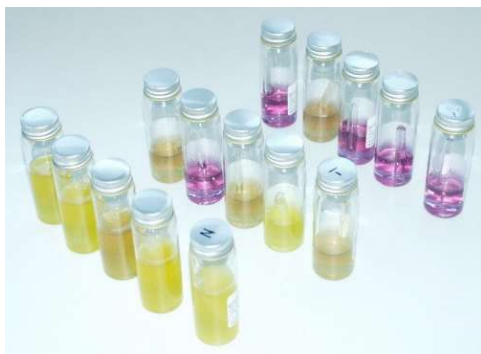
Figure 2. MMGM at three dilutions after incubation showing change of colour
