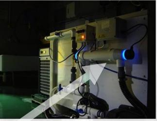
Figure 1 UV steriliser unit (adapted from Seafish technical report)
