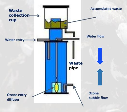
Ozone bubbles introduced at the bottom of the skimmer strip the water of impurities which cling to them by surface tension
