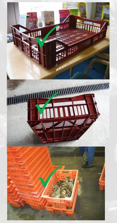
Containers used to hold live bivalve molluscs in purification systems must have a construction that allows clean seawater to flow through
