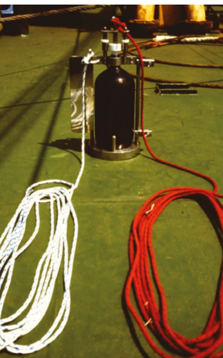
Figure 1. Cefas sub-surface water sampler rigged for use. The sampler is lowered using the white rope, and opened and closed using the red rope. Note the clips and stabilising vane for deployment from a hydro-wire
