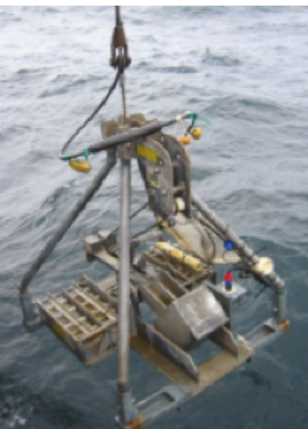
Figure 7. Mini-Hamon grab (fitted with video system), the combined gear being known as HamCam.
